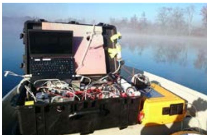
*The portable mass spectrometer on Soppensee (Switzerland). Photo: EAWAG – Swiss Federal Institute of Aquatic Science and Technology*
