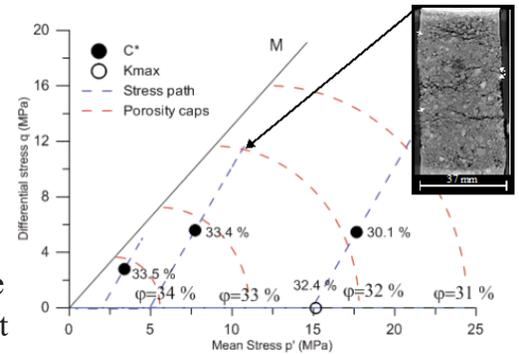
*Porosity reduction predicted from hydrostatic loading using an end-cap model and experimental measured porosity reduction for the onset of shear-enhanced compaction, C\*, during axial loading. Inserted is a micro CT scan showing sample deformation at the end of the 5 MPa confining pressure test on uncemented sandstone.*
